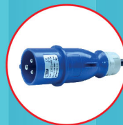
Industrial Power Plug IEC 60309, IP44 (16A & 32A)
